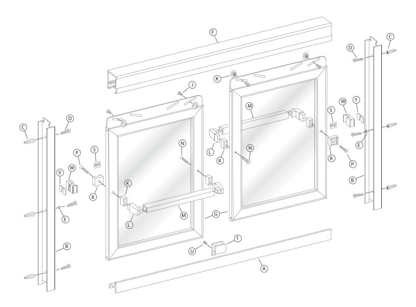
Measure the wall to wall opening at the center of the threshold. Cut the bottom track [A] 1/16" short of that dimension. An inexpensive miter box (available at a hardware store) will help you get a clean, square cut.
