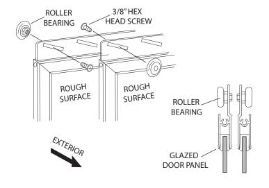
The Lift the interior panel (textured side of glass on the same side as the top fin) into position with the rollers engaging the roller track in the header.
