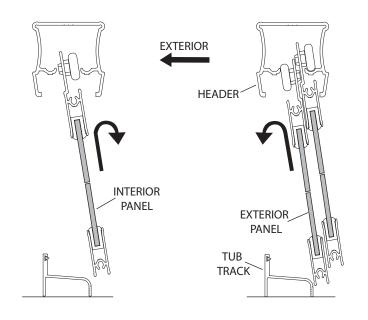
Before finishing the installation, it is necessary to determine the proper closed position of the door panels. For maximum water control, position the interior panel closest to the shower head. (see illustration)
