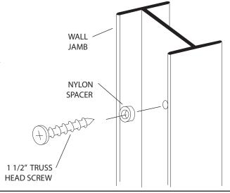
5 This enclosure is equipped with safety "T" lock wall jambs. When properly installed, the header is permanently locked to the wall jambs and cannot be accidently dislodged.
