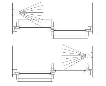
9 Slide the four metal towel bar trim rings [K] over the clear acrylic towel bar brackets [L]. Press the brackets into the ends of the two towel bars [M].
