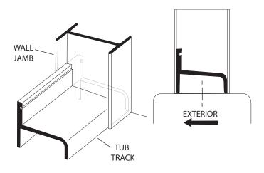
2 Using a level, plumb one wall jamb and mark the three hole locations on the wall with a pencil. Repeat this step for the other wall jamb. Remove all parts and drill the holes.
