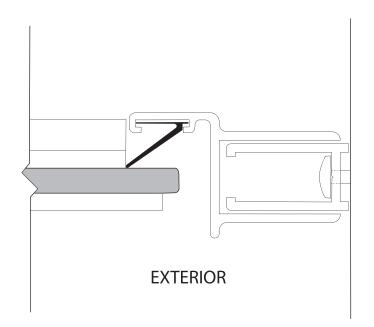
12 Carefully silicone the seam between the wall and the wall jamb as well as the curb and threshold on the inside of the shower.
