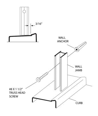
4 Measure the finished wall-to-wall opening at the top and bottom of the wall jambs. Note the smaller dimension (see bottom left illustration).
