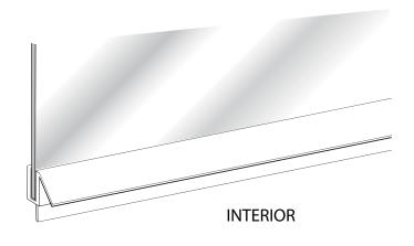
11 Place the sweep onto the bottom of the door. Stand inside the shower, close the door and mark the deflector part of the sweep at the inside edge of the strike jamb.
