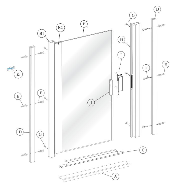
1 The 3610 Continuous Hinge Shower Door is completely reversible and may be installed hinge-right or hinge-left. Refer to the illustration to determine the best hinge position for your installation. For maximum waterproofing, the hinge jamb should always be opposite the shower head. The following instructions depict a hinge-left installation.
