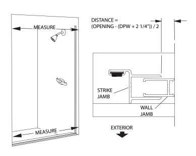
Inside the shower enclosure, using the pencil marks on the wall jambs from the previous step, drill two 1/8" holes through the strike jamb [H] and into the wall jamb [D] 3/8" to 3/4" from the wall and approximately 1" down from the top and up from the bottom of the strike jamb. Drill a third hole centered between the first two.
