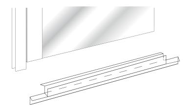
10 Align the clear bottom sweep to the bottom of the door with the deflector lip on the inside of the shower door. Mark the strike side of the bottom sweep even with the strike edge of the door. Cut the sweep leaving the notched part under the metal rail.
