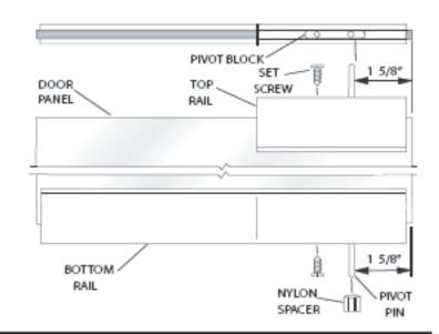
Insert the two nylon pivot bushings [AA] into the pivot holes in the head and curb fillers [P].
