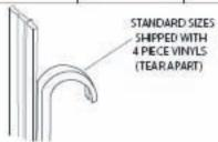
Cut eight pieces of the smaller vinyl [JJ] 1" longer than the vertical opening (to prevent gapping from shrinkage) and trim the ends on a 45° angle. Using the masking tape guides, center the first glass panel [J] in the frame. Cut four short (1" – 2") pieces of the small vinyl and press into the jamb and post on each side to hold the glass temporarily.
