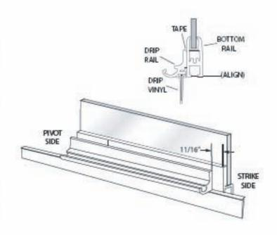
Adjust the drip vinyl [V] by sliding it left or right until it almost touches the curb. Trim the vinyl (flush with the pivot end and notch 1/2" longer than the drip rail as shown on the strike end). Secure it with one #6 x 3/8" truss head screw [FF] in the pivot end of the drip rail [T].
