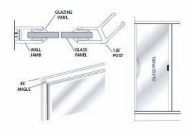
Cut eight pieces of the larger vinyl [KK] 1/2" longer than the horizontal opening and trim the ends on a 45° angle. Install the top exterior vinyl starting at both ends and working toward the middle. Be careful not to stretch the vinyl.
