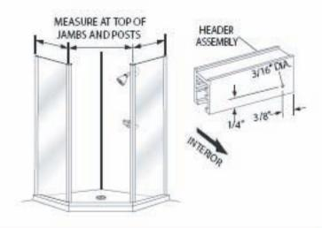
Press the header assembly [D] over the wall jambs [E] and 135° posts [K]. Check the posts for plumb. Adjust as required by varying the overlap of the header over the wall jambs. You may need to trim the ends of the header where it meets the wall. The minimum horizontal dimension for the door opening is the door panel width (see the graphic in Step #9) plus 1/2", maximum is the door panel width plus 1 3/4".
