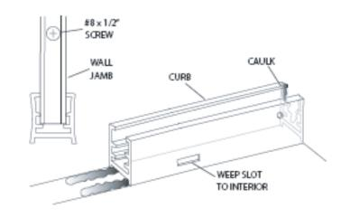
Place the setting blocks [H] in the curb assembly [A] as shown to support the two fixed glass panels [J]. Positioned the blocks 3" from the comer of the panels. Set the first glass panel into place on the setting blocks and approximately 1/2" into the wall jamb [E]. A strip of masking tape 1/2" from each vertical edge of the glass will aid alignment.
