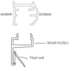
**8** Pull the top of the hinge jamb (H) tight with the snap-n-fill (J) use a level to make sure the door panel is plumb.
