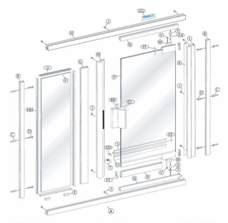
The BASCO 136/736 Thin-Line Shower Enclosure is completely reversible and may be installed pivot-left or pivot-right. The door may pivot from the wall or from the center post. For maximum waterproofing, the pivot jamb should be opposite the showerhead. Using the illustration, determine the correct position for the door in your particular Thin-Line installation. This instruction sheet depicts a pivot-right installation.
