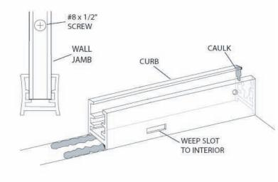
**5** Place two setting blocks [**E**] into the curb [**A**] to support the fixed glass panel [**F**]. Position the blocks 3" from each corner of the glass panel. Set the glass panel into place on the setting blocks and approximately 1/2" into the wall jamb [**B**]. A strip a masking tape 1/2" from each vertical edge of the glass will aid alignment.
