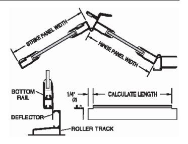
9 Slide the pivot block located in the bottom rail of the strike door panel as close to the leading edge of the panel as it can go. Install the headless pivot pin screw [L] into the pivot block and tighten securely. Do not over-tighten or deform the head of the pivot pin screw.
