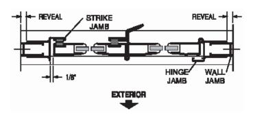
Inside the shower enclosure, align the slots on the hinge jamb with the holes in the wall jamb [E]. Start a #8 x 3/8" truss head screw [M] in the bottom slot and hole but do not tighten it completely. Pull the top of the hinge jamb outward until there is 1/8" clearance between the roller track and the bottom of the strike door panel. Hold the hinge jamb in this position while installing a second #8 x 3/8" screw in the top slot and hole. Install a third screw in the center slot and hole.
