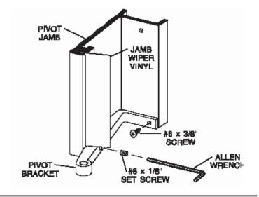
Place the pivot jamb [C] on the curb [A] with the exterior face lined up with the raised edge of the curb. Use a level to plumb the jamb then mark the mounting hole locations. Remove the jamb and drill the mounting holes.
