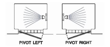
Note: The 100/200 unit may be installed without using the sloped curb [A] provided. Its use is definitely recommended for positive water control on shower sills with little or no slope.
