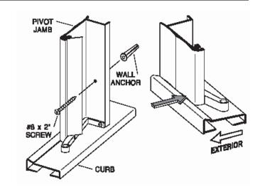
Replace the pivot jamb and attach to the wall with three  $\#8 \times 2$ " truss head screws [K].
