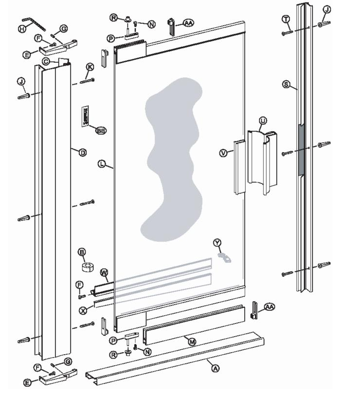
The Basco 3600 Frameless Pivot Shower Door is completely reversible and may be installed pivot-right or pivot-left. Refer to the illustration to determine the correct position for your installation. For maximum waterproofing, the pivot jamb should always be opposite the shower head. These instructions depict a pivot-left installation.
