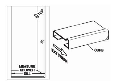
Run two beads of caulk along the flat surfaces on the bottom of the curb [A]. Then replace the curb on the shower sill in the exact position marked in Step #2. Press firmly into place with the raised portion to the exterior of the enclosure.
