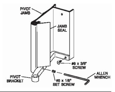
Place the pivot jamb assembly on the curb [A] with the exterior face lined up with the raised edge of the curb. Use a level to plumb the jamb then mark the mounting hole locations. Remove the jamb and drill the mounting holes.
