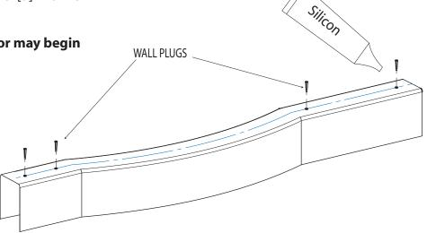
**5** Using the u-channel [B1/B2] of lengths 71-1/4" & 73-1/4". Place the u-channel [B1] of length 71-1/4" on the higher wall. Cut the second piece of u-channel [B2] according to the out of level conditions (See Picture).
