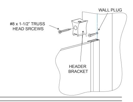
**9** Place the corner vinyl [U] on the exposed corners of the glass. Now place the corner header brackets [N] over the corner vinyl [U].
