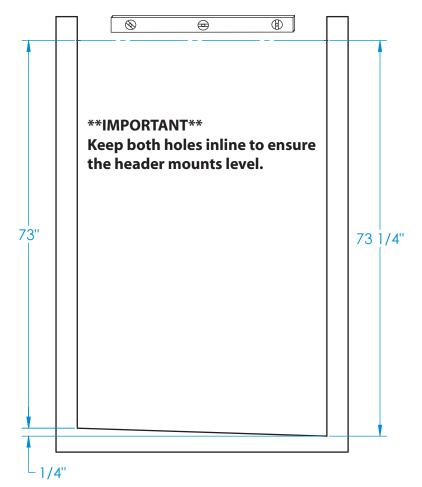
**3** Using U-channel [B3] of length 34", cut two pieces to the appropriate sizes. Each piece will be equal to it's respective panel width referenced in Step1 ("a" and "b").
