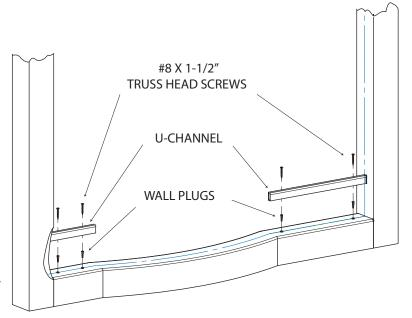
Insert a small amount of silicon into each hole, then insert a wall plug [V] in each hole. (Note: This must be done just before u-channel installation.) Then carefully cut heads off wall plugs [V] with a razor blade. Place each u-channel in correct position and secure each piece of u-channel [B] with #8 x 1-1/2" truss head screws [X].
