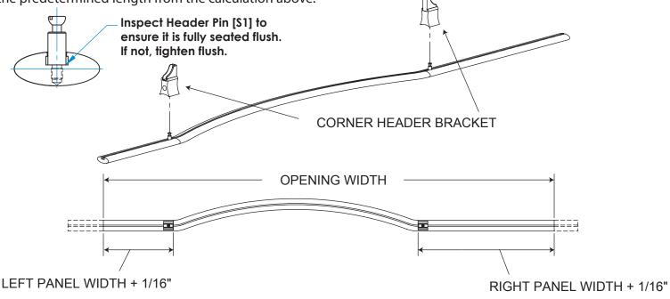
Take both header brackets [O] and drill 3/16" hole completely through the end. Next put a wall plug [V] into the hole that was drilled in the wall, and silicon the wall plug [V]. Then carefully cut heads off wall plugs. Place the header bracket [N] back onto the vertical u-channel [B] and screw into the wall with the #8 x 1-1/2" set screws [X]. Repeat this process on each side of enclosure.
