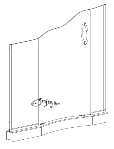
16 The door is best installed with two people. Position one person on each side of door panel and carefully place the door panel over the hinge notches. As the person to the outside of the door holds the door panel, the other person installs the hinge back plates, gaskets, and screws. To complete installation. Now repeat the same process for each hinge.
