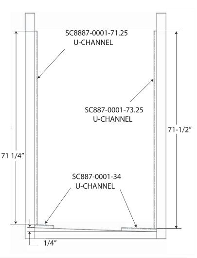
Place a small amount of silicon into each hole and insert a wall plug [V]. (Note: This must be done just before u-channel installation.) Then carefully cut heads off wall plugs [V] with a razor blade. Place u-channel [B] in correct position and secure each piece of u-channel [B] with #8 x 1-1/2" truss head screws [X].
