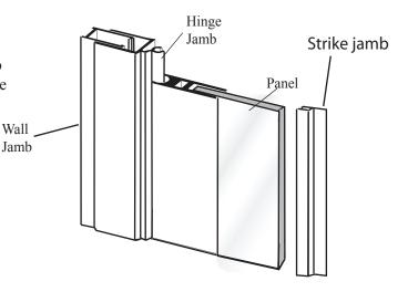
**7**When installing the 2nd panel slide the hinge jamb of the door panel assembly (H) over the mounted wall jamb (B) so the door will open outward while holding the panel, install the snap-n-fill (J) into the header. This will allow you to adjust the 2nd door.
