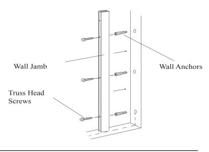
**3** Measure the wall-to-wall opening at the top of the wall jambs [**B**] and cut the header [**E**] to fit the exact opening. Using a 1/8" drill bit, drill the interior face of the header on both ends as shown.
