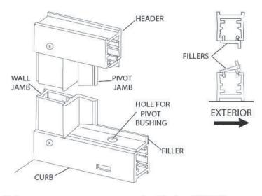
**10** Pull the bottom of the pivot jamb [L] tight to the curb filler [N] and plumb the jamb. Drill two 1/8" holes thru the pivot jamb and into the wall jamb [B] 3/8" to 3/4" from the wall and approximately 1/4" from the ends of the jamb. Drill a third hole centered between the first two, then enlarge the three outer holes with a 3/16" drill for clearance on the self-tapping screws. Attach the pivot jamb permanently with three #8 x 1/4" truss head screws [J].
