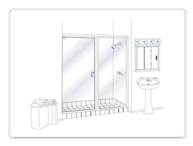
**MAINTENANCE:** Two primary materials are used to manufacture your new Basco enclosure: tempered glass and anodized aluminum. To assure a long lasting finish on the enclosure, wipe it down with a towel after each use. Never use a scouring agent to clean the aluminum.
