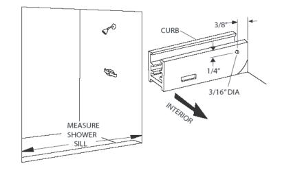
Place the two wall jambs [**B**] into the ends of the curb [**A**]. Masking tape may be used to hold the curb in place during this operation. Plumb the jambs and mark the hole locations on the wall. Remove all parts and drill the walls for mounting hardware.
