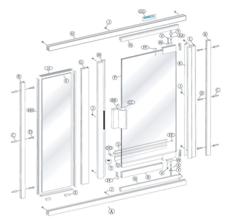
The BASCO 136/736 Thin-Line Shower Enclosure is completely reversible and may be installed pivot-left or pivot-right. The door may pivot from the wall or from the center post. For maximum waterproofing, the pivot jamb should be opposite the showerhead. Using the illustration, determine the correct position for the door in your particular Thin-Line installation. This instruction sheet depicts a pivot-right installation.
