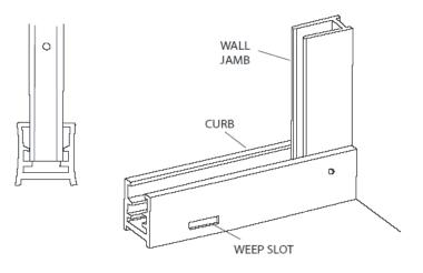
**4** Wipe the shower walls and sill, curb [**A**] and wall jambs [**B**] with a clean, dry cloth to remove any dust or debris. Apply a 1/4" bead of caulk along the inside of both of the pencil lines marked in Step #2. Carefully replace the curb in the exact position marked. Caulk the inside of the curb ends where they meet the wall.
