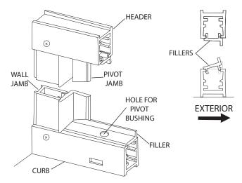
Pull the bottom of the pivot jamb [M] tight to the curb filler [P] and plumb the jamb. Drill two 1/8" holes thru the pivot jamb and into the wall jamb [B] 3/8" to 3/4" from the wall and approximately 1/4" vertically from the ends of the jamb. Drill a third hole centered between the first two and enlarge the outer holes with a 3/16" drill for clearance on the self-tapping screws. Attach the pivot jamb permanently with three #8 x 1/4" truss head screws [J].
