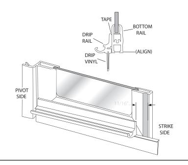
Adjust the drip vinyl [T] by sliding it left or right until it almost touches the curb. Trim the vinyl (flush with the pivot end and notch 1/4" longer than the drip rail as shown on the strike end).
