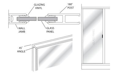
Cut four pieces of the larger vinyl [FF] 1/2" longer than the horizontal opening and trim the ends on a 45° angle. Install the top exterior vinyl starting at both ends and working toward the middle. Be careful not to stretch the vinyl.
