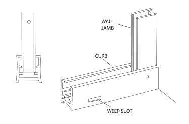
Wipe the shower walls and sill, curb [A] and wall jambs [B] with a clean, dry cloth to remove any dust or debris. Apply a 1/4" bead of caulk along the inside of both of the pencil lines marked in Step #2. Carefully replace the curb in the exact position marked. Caulk the inside of the curb where it meets the wall.
