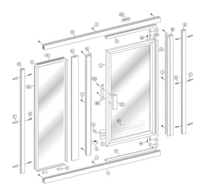
The BASCO 135/735 Thin-Line Shower Enclosure is completely reversible and may be installed pivot-left or pivot-right. The door may pivot from the wall or from the center post. For maximum waterproofing, the pivot jamb should be opposite the showerhead. Using the diagram, to determine the correct position for the door in your particular installation. This instruction sheet depicts a pivot-right installation.
