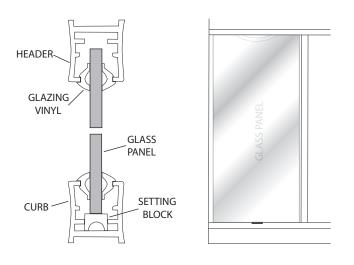
Carefully caulk the interior jamb-to-wall and curb-to-base joints. For appearance, you may wish to caulk the exterior joints as well. We recommend you wait twenty-four hours before the first shower to allow the caulking to cure properly.
