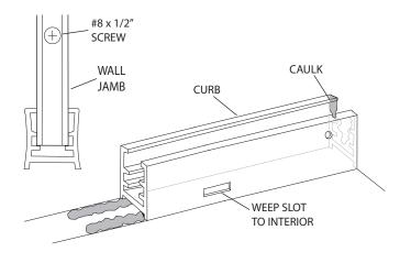
Place the setting blocks [E] in the curb [A] as shown to support the fixed glass panel [F]. The setting blocks should be positioned approximately 3" from each corner of the glass panel. Remove any protective strips from the glass panel and set it into place. It should rest on the setting blocks and be engaged approximately 1/2" into the wall jamb [B]. A strip a masking tape 1/2" from each vertical edge of the glass will aid alignment.
