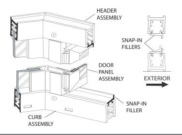
**10** Pull the hinge jamb tight against the snap-in fillers forcing them to sit tight to the strike jamb. There should be a 1/8" clearance between the strike jamb and the edge of the strike jamb with the door being in the closed position.
