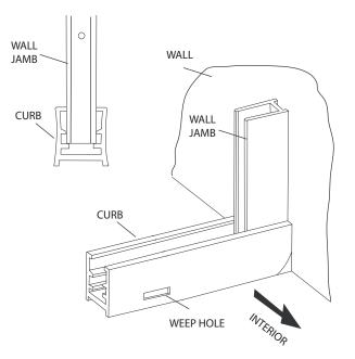
**4** Wipe the shower walls, sill, curb & wall jambs with a clean, dry cloth to remove any dust or debris. Apply a 1/4" bead of silicone along the inside of the pencil lines that were marked in Step #2. Carefully place the curb on the sill, over top the silicone, in the position marked.
