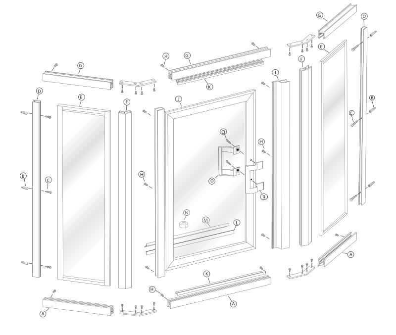
The 675 Quick N' Stall Neo Angle Framed Hinge Shower Enclosure is completely reversible and may be installed hinge right or hinge left. For maximum leak protection, the hinge side should be opposite the shower head. Using the illustration, determine the proper hinge side for the door.
