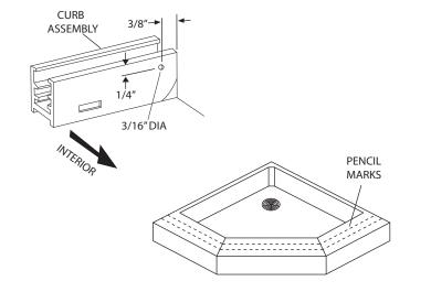
**3** Place one wall jamb [**D**] into the curb against the wall. Using a level, plumb the wall jamb and mark the hole locations on the wall with a pencil. Repeat this step for the other wall jamb. Remove all parts and drill the holes.
