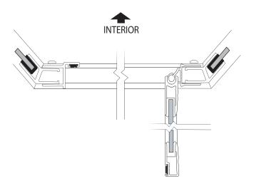
9 Keeping the door in the open position, press the snap-in fillers [K] into the curb and header between the hinge and strike jambs. BE SURE THE RAISED LIP IS TO THE EXTERIOR (see illustration).
