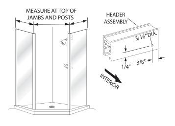
Press the header assembly **[G]** over the wall jambs, 135° posts and pre-glazed return panels. Check the posts for plumb. Adjust as required by varying the overlap of the header and wall jambs. You may need to trim the ends of the header where it meets the wall.
