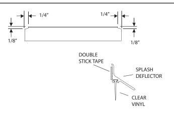
**12** Position the deflector so that the bottom of the vinyl is 1/16" from the curb, and the deflector is 1/16" from the continuous hinge jamb. (see illustration)
