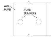
**10** Neatly silicone each end of the tub track where it fits into the wall jambs as well as the seam between the wall and the wall jamb and the curb and threshold on the inside of the shower.
