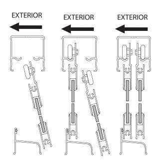
NOTE: Be sure that there is enough space under the inside door panel for it to clear the bottom guide.
