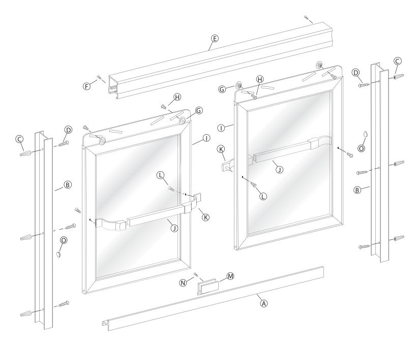
Measure the wall-to-wall opening at the center of the tub rim. Cut the tub track [A] 1 1/8" short of this dimension. An inexpensive miter box (available at your local hardware store) will help you get clean square cuts.
