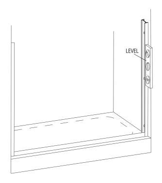
Before replacing the tub track, gently force a slight bow in the part so that the middle will sit on the threshold and both sides are slightly raised. (This will ensure that the track fits tight to the threshold when installed)
