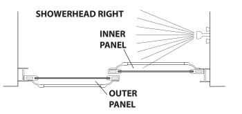
Slide both panels to one side of the opening. Center panel guide [M] on the track under interior door panel as shown. Using the hole in the panel guide, drill a 1/8" hole into the track.
