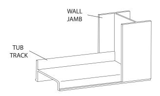
Place one wall jamb [B] against the wall and inside the open space between the curb. Using a level, plumb the wall jamb and mark the hole locations on the wall with a pencil. Repeat this step for the other wall jamb. Mark along both inside and outside of the track.
