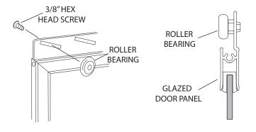
Place one door panel [I] on the inside of the tub/shower with the rollers facing the back wall and the textured side of the panel facing the outside (if applicable). Set it on a drop cloth or piece of cardboard to protect the tub/shower surface from the metal corners.
