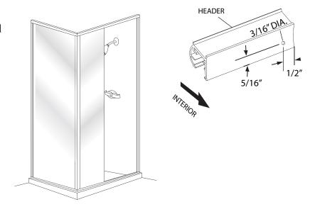
**8** Press the header assembly over the wall jambs and corner post (if applicable). Check both sides of the post for plumb. Adjust as required by varying the overlap of the header over the wall jambs.
