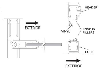
\*\* Prior to installation, be sure that the magnet [P] and vinyl [Q] are inserted into the flange. The open part of the vinyl should be facing down and the magnet should be on the side closest to the stationary panel.
