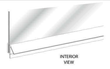
22 Place the sweep back onto the bottom of the door. Step inside the shower and close the door. Mark on the sweep at the edge of the polycarbonate strike jamb.
