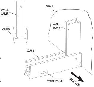
Wipe the shower walls, sill, curb & wall jambs with a clean, dry cloth to remove any dust or debris. Apply a 1/4" bead of silicone along the inside of the pencil lines that were marked in Step #2. Carefully place the curb on the sill, over top the silicone, in the position marked.
