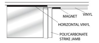
18 Fold the vinyl material [S] over the top edge of the glass lining it up with the magnet. Mark the two ends of the magnet onto the vinyl with a pencil. Carefully drive the latch [T] onto the door panel using a rubber or plastic mallet.
