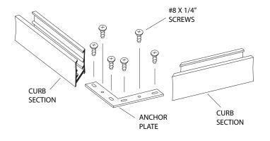
Assemble the two header sections [C] in the same manner.
