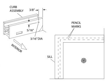
Place one wall jamb [D] into the curb against the wall. Using a level, plumb the wall jamb and mark the hole locations on the wall with a pencil. Repeat this step for the other wall jamb. Remove all parts and drill the holes. TIP: Tape can be used to temporarily hold the curb in place.
