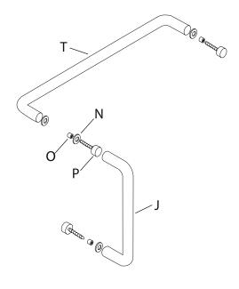
J Exterior handle (1) T Towel bar (1) N SC4586 Small clear discs (6) O SC4587 Glass hole sleeve (3)
