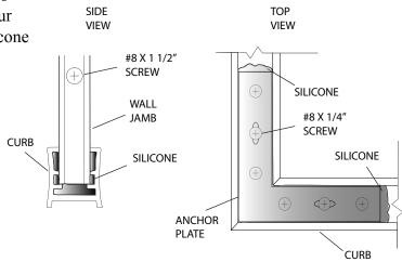
Place four setting blocks [G] into the curb, flat side up, to support the stationary glass panels. Position the blocks so they are centered about 3" from each corner of the glass panel. Set the return glass panel [H] in the curb on the setting blocks and slide into the wall jamb approximately 1/2".
