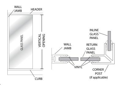
**Caution:** Do not to stretch the vinyl when pressing into place and keep the glass pushed against the snap-in fillers.
