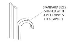
10 Once the panels are set in place, cut four small pieces of the horizontal [L] (crescent shaped) vinyl about 3" and install them into the header and curb (open side of the crescent shape against the glass). This will help hold the panel in place while installing the door panel.
