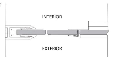
22 Carefully silicone the seam between the walls and the wall jambs as well as the curb and threshold on the inside of the shower.
