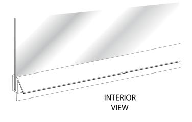
21 Place the sweep back onto the bottom of the door. Step inside the shower and close the door. Mark on the sweep at the edge of the polycarbonate strike jamb.
