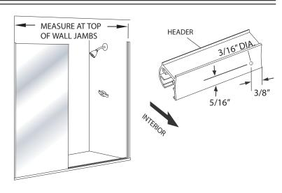
7 Slide the header over the wall jambs. Using the two holes on the interior face of the header as a guide, drill a 1/8" hole into each wall jamb. Attach the header to the wall jambs using two #8 x 1/4" Truss Head screws [H].
