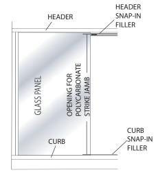
16 Remove the magnet and slide the vinyl partially out of the header snap-in filler. Trim enough of the vinyl so that the magnet is not covered by the lip of the polycarbonate strike jamb (approximately 3/8" should suffice). Slide the vinyl back into the filler and replace the magnet. Place a small amount of silicone at the end of the magnet to hold in place.
