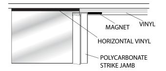
17 Fold the vinyl material [Q] over the top edge of the glass lining it up with the magnet. Mark the two ends of the magnet onto the vinyl with a pencil. Carefully drive the latch [R] onto the door panel using a rubber or plastic mallet.
