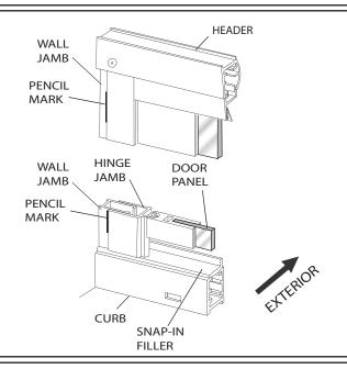
Verify that the door has not shifted using the pencil marks. Then, from the inside of the enclosure, drill two 1/8" holes through the hinge jamb and into the wall jamb approximately 1" from the ends of the jambs at the top and bottom and 3/16" from the edge of the open side of the hinge jamb. (see illustration)
