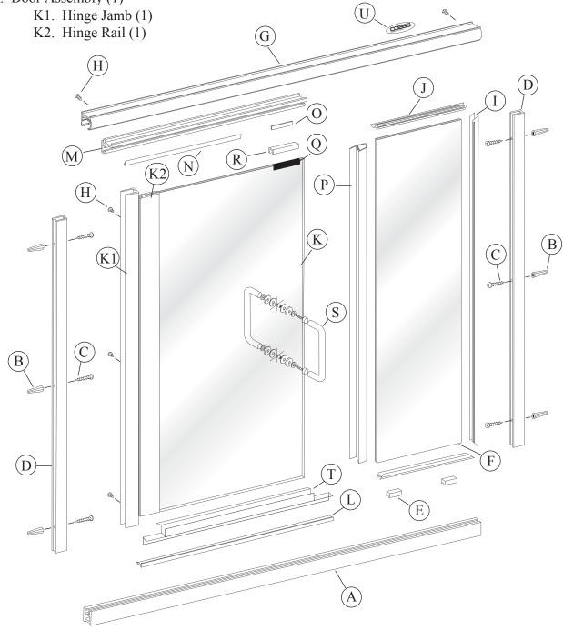
The Basco 1413NP / 1713NP / 1813NP Frameless Continuous Hinge Shower Enclosure must be installed with the door hinged off of the wall. It may be installed hinge right or hinge left. But, for maximum leak protection, the hinge side should be opposite the shower head. Using the illustration, determine the proper hinge side for the door. Careful as to not follow the illustrations exactly.
