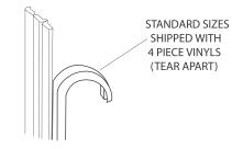
Once the panel is set in place, cut four small pieces of the horizontal [J] (crescent shaped) vinyl about 3" and install them into the header and curb (open side of the crescent shape against the glass). This will help hold the panel in place while installing the door panel.
