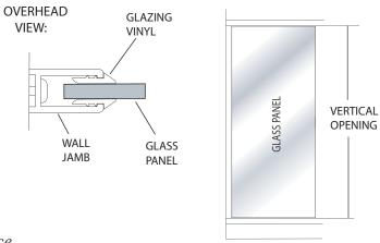
**Caution:** Do not to stretch the vinyl when pressing into place and keep the glass pushed against the snap-in fillers.
