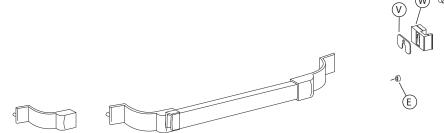
Measure the wall-to-wall opening at the center of the tub rim. Cut the tub track [B] 1 1/8" short of this dimension. An inexpensive miter box (available at your local hardware store) will help you get clean square cuts.
