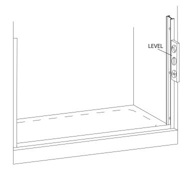
Before replacing the tub track [A], gently force a slight downward bow in the extrusion. This will ensure the track fits tight to the tub. Caulk the bottom legs of the tub track as shown and replace in the exact position marked in Step #2.
