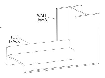
**2**Use a level to plumb both wall jambs [B] and mark the pre-drilled hole locations on the wall. Lightly mark along both sides of the tub track [A] with a pencil and remove all parts.
