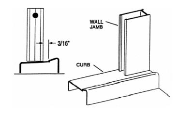
Slide the strike jamb [**F**] over one of the mounted wall jambs [**B**] with the magnet facing outward.
