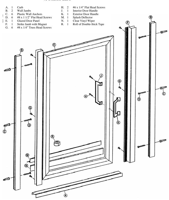
The Basco 75 Continuous-Hinge Shower Door is completely reversible and may be installed hinge-left or hinge-right. Refer to the illustration to determine the correct position for your installation. For maximum waterproofing, the hinge jamb should always be opposite the shower head. These instructions depict a hinge-left installation.
