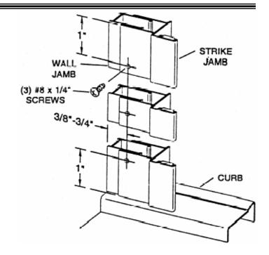
Slide the door panel [E] over the other wall jamb [B] until the door panel and the strike jamb [F] can meet. With the door closed and the latch magnets engaged, the proper door panel to strike jamb clearance is 1/8" (see illustration). Mark the hinge jamb's location on the wall jamb with a pencil.
