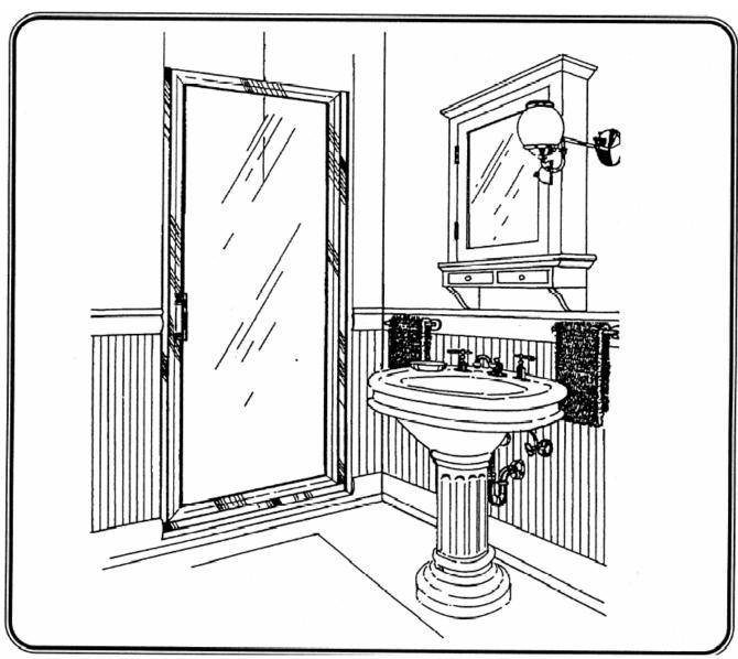
**MAINTENANCE:** Two primary materials are used to manufacture your new Basco enclosure: tempered glass and anodized aluminum. To assure a long lasting finish on the enclosure, wipe it down with a towel after each use. Never use a scouring agent to clean the aluminum.
