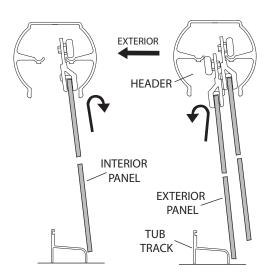
Locate the nylon bottom guide [S] in the middle of the tub track [A] with the glass panels in the position shown. With a 7/64" bit, drill two holes into the V-groove through the mounting holes in the guide. Install the bottom guide with two #6 x 3/8" pan head screws [T] thru the drilled holes as shown.
