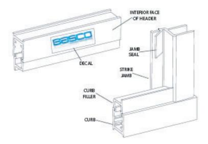
Inspect the pieces of black glazing vinyl, and note the two different profiles. The smaller shape [JJ] is installed vertically and the larger shape [KK] is installed horizontally. For structural strength and maximum water resistance, these vinyls are designed to fit tightly between the glass and framing. To speed installation, use glass cleaner for lubrication and a small block of wood to press the vinyl into place.
