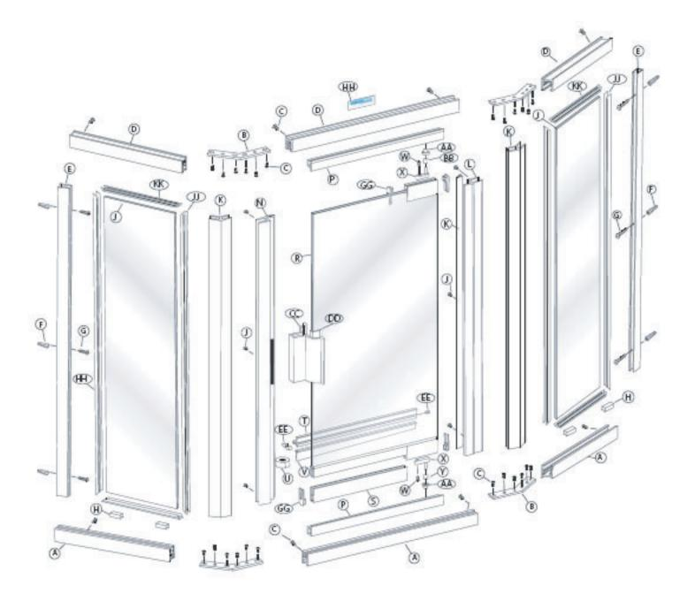
The BASCO 161/761 Thin-Line Shower Enclosure is completely reversible and may be installed pivot-left or pivot-right. For maximum waterproofing, the pivot jamb should be opposite the shower head. Use the diagram to determine the correct position for the door in your particular Thin-Line installation. This instruction sheet depicts a pivot-right installation.
