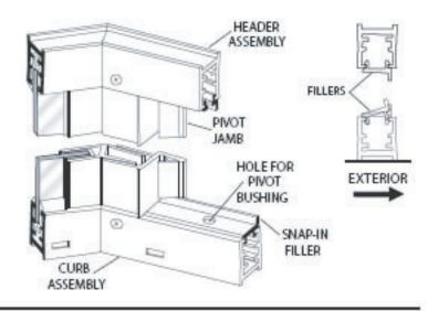
Pull the bottom end of the pivot jamb [M] tight to the curb filler [P] and plumb the jamb. Drill two 1/8" holes thru the pivot jamb and into the 135° post [K] in line with the screws in the head and curb and approximately 1/4" from the ends of the jamb. Drill a third hole centered between the first two, then enlarge the outer holes with a 3/16" drill for clearance on the self-tapping screws. Attach the pivot jamb permanently with three #8 x 1/4" truss head screws [C].
