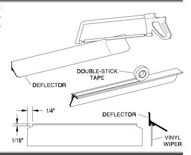
Hold the splash deflector [P] against the inside of the door bottom rail 1/16" from the hinge jamb and with the vinyl wiper [R] just touching the curb. Mark the location of each end of the deflector with a pencil. Peel the backing off of the double-stick tape [S] and carefully (you only get one try) stick the splash deflector to the door using the marks for alignment.
