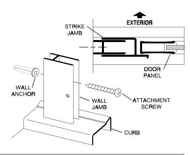
Slide the adjustable strike jamb outer portion [**E**] over the inner wall jamb portion [**F**]. Adjust the outer jamb laterally to provide 1/8" to 3/16" clearance between the door panel and the strike jamb.
