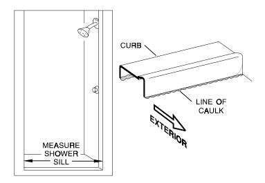
Place the door panel/hinge jamb assembly [B] in place on the curb [A] with the hinge jamb lined up with the raised edge of the curb. Use a level to plumb the jamb, then mark the mounting hole locations. Remove the door assembly and drill the mounting holes.
