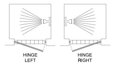
NOTE: The 15/16 unit may be installed without using the sloped curb [A] provided. Its use is definitely recommended for positive water control on shower sills with little or no slope.
