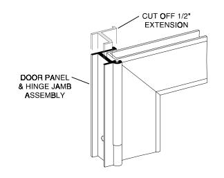
Set the door panel/hinge jamb assembly [**B**] back onto the curb [**A**] and attach it securely with three #8 x 1 1/2" flat head screws [**D**] through the hinge jamb.
