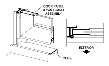
To allow this unit to be reversible, the hinge jamb extends 1/2" beyond both ends of the door panel. Once the proper door orientation has been determined (see Step #1), the 1/2" extension at the *top* of the door can be cut off for better appearance.
