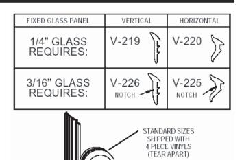
Cut four pieces of the smaller vinyl [FF] 1" longer than the vertical opening (to prevent gapping from shrinkage) and trim the ends on a 45° angle. Using the masking tape guides, center the first glass panel [J] in the frame. Cut four short (1"-2") pieces of the small vinyl and press into the jamb and post on each side to hold the glass temporarily.
