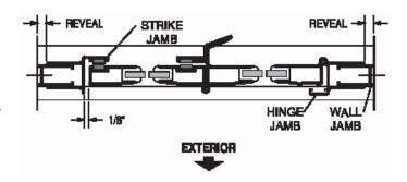
Inside the shower enclosure, align the slots on the hinge jamb with the holes in the wall jamb [E]. Start a #8 x 3/8" truss head screw [M] in the bottom slot and hole but do not tighten it completely. Pull the top of the hinge jamb outward until there is 1/8" clearance between the roller track and the bottom of the strike door panel. Hold the hinge jamb in this position while installing a second #8 x 3/8" screw in the top slot and hole. Install a third screw in the center slot and hole.
