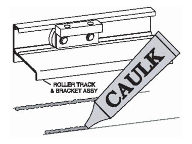
Run two beads of caulk inside the penciled marks on the shower sill. Place the roller track [A] (with roller bracket) in the exact position marked in Step #2 and seat it firmly in the caulking. Use masking tape to temporarily secure roller track.
