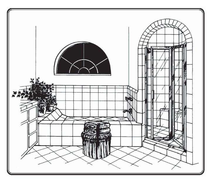
**MAINTENANCE:** Two primary materials are used to manufacture your new Basco enclosure: tempered glass and anodized aluminum. To assure a long lasting finish on the enclosure, wipe it down with a towel after each use. Never use a scouring agent to clean the aluminum.
