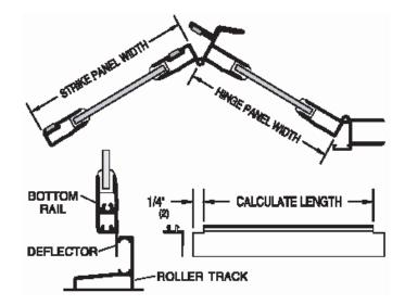
Slide the pivot block located in the bottom rail of the strike door panel as close to the leading edge of the panel as it can go. Install the headless pivot pin screw [L] into the pivot block and tighten securely. Do not over-tighten or deform the head of the pivot pin screw.
