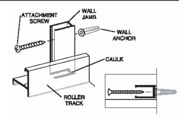
Drill two 7/64" diameter holes through the roller track [A] and into the wall jambs 1/4" from the top of the curb and 3/8" from the wall. Secure the roller track to the wall jambs with two #5 x 1/2" screws [H].
