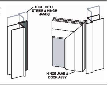
Measure the bottom rails of the strike and hinge door panels to determine the panel widths. Cut one section of the clear vinyl splash deflector [N] 2" shorter than the width of the strike panel. Trim the second section 3/8" longer than the hinge panel. Notch ends of both deflectors as shown, leaving only the thin vertical portion extending. Snap the deflectors into the bottom rail of their respective door panels.
