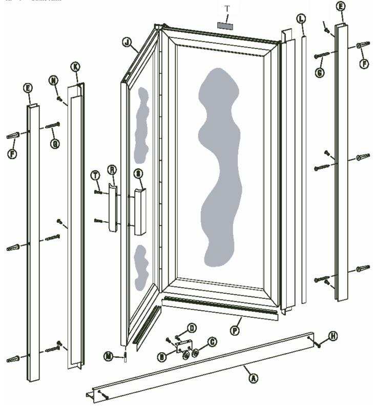
The Basco 1100 Bi-fold Shower Door is completely reversible and may be installed hinge-right or hinge-left. Using the diagram, determine the correct position for your installation. For maximum waterproofing, the pivot jamb should always be opposite the showerhead. These instructions depict a hinge-right installation.
