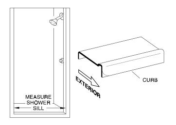
Run two beads of caulk inside the penciled marks on the shower sill. Place the curb [A] in the exact position marked in Step #2 and seat it firmly in the caulking.
