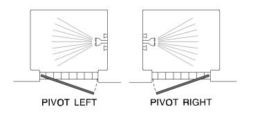
NOTE: The 100/200 unit may be installed without using the sloped curb [A] provided. Its use is definitely recommended for positive water control on shower sills with little or no slope.
