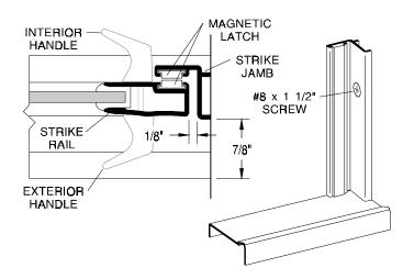
Attach the interior door handle [ $\mathbf{R}$ ] and the exterior door handle [ $\mathbf{S}$ ] to the door with two #6-32 x 1 1/4" round head screws [ $\mathbf{T}$ ].
