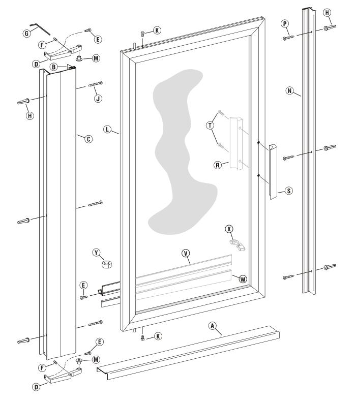
The BASCO 100/200 Pivot Shower Door is completely reversible and may be installed pivot-right or pivot-left. Using the diagram, determine the correct position for your installation. For maximum waterproofing, the pivot jamb should always be opposite the shower head. These instructions depict a pivot-left installation.
