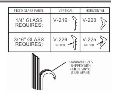
**18** Cut eight pieces of the smaller vinyl [FF] 1" longer than the vertical opening (to prevent gapping from shrinkage) and trim the ends on a 45° angle. Using the masking tape guides, center the first glass panel [J] in the frame. Cut four short (1" - 2") pieces of the small vinyl and press into the jamb and post on each side to hold the glass temporarily.
