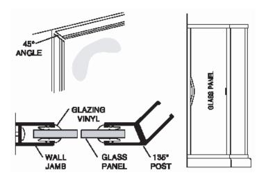
Cut eight pieces of the larger vinyl [GG] 1/2" longer than the horizontal opening and trim the ends on a 45° angle. Install the top exterior vinyl starting at both ends and working toward the middle. Be careful not to stretch the vinyl.
