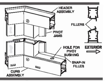
Pull the bottom end of the pivot jamb [N] tight to the curb filler [R] and plumb the jamb. Drill two 1/8" holes thru the pivot jamb and into the  $135^{\circ}$  post [K] in line with the screws in the head and curb and approximately 1/4" vertically from the ends of the jamb. Drill a third hole centered between the first two, then enlarge the outer holes with a 3/16" drill for clearance on the self-tapping screws. Attach the pivot jamb permanently with three #8 x 1/4" truss head screws [C].
