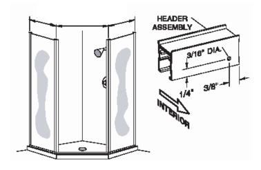
**8** Press the header assembly **[D]** over the wall jambs **[E]** and 135° posts **[K]**. Check the posts for plumb. Adjust as required by varying the overlap of the header over the wall jambs. You may need to trim the ends of the header where it meets the wall. The minimum horizontal dimension for the door opening is the door panel width (see the graphic in Step #9) plus 1/2", maximum is the door panel width plus 1 3/4".
