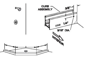
Place the two wall jambs [E] into the ends of the curb assembly [A]. Masking tape may be used to hold the curb in place during this operation. Plumb the jambs and mark the hole locations on the wall. Remove all parts and drill the walls for mounting hardware.
